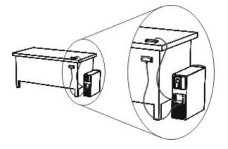
2. Insert the receiver's captive USB cable connector into an available USB receptacle on your computer.
